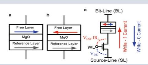
Parallel (Low basics: (a) STT-RAM Resistance). (b) Anti-parallel (high Resistance) (c) 1T1MTJ cell structure [Weisheng Zhao, 2015]
