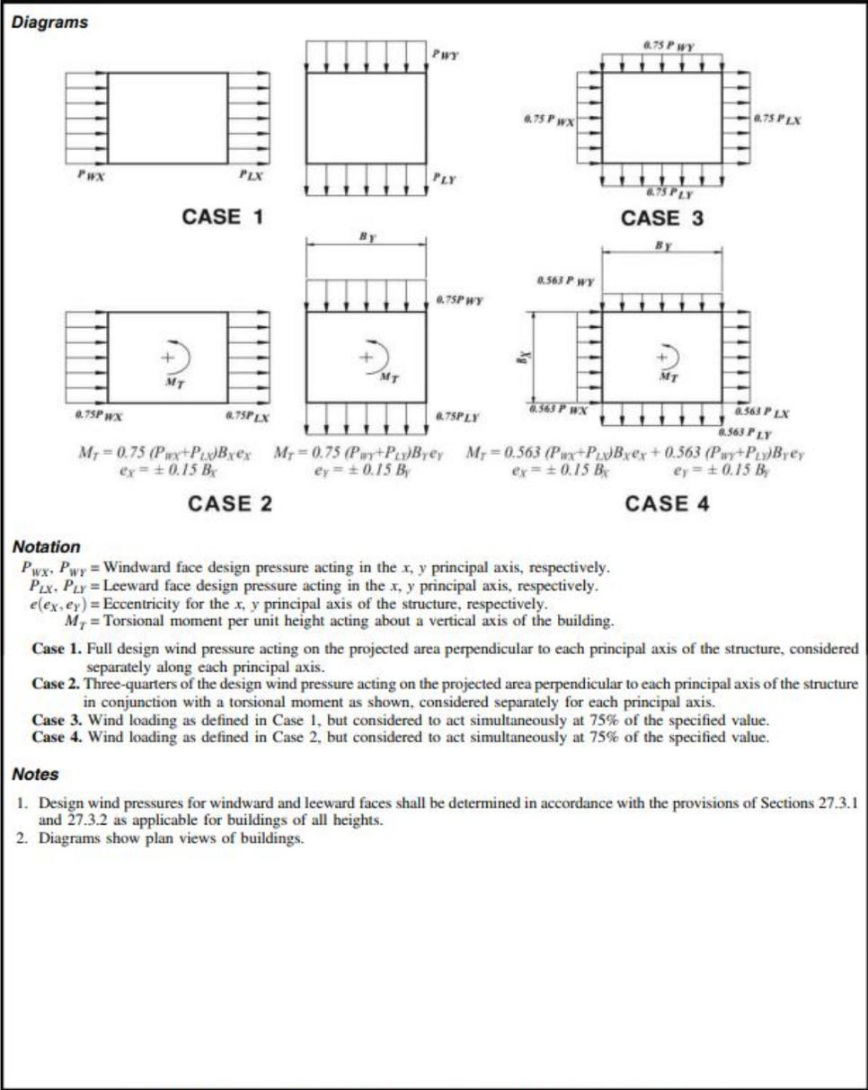
FIGURE 27.3-8 Main Wind Force Resisting System, Part 1 (All Heights): Design Wind Load Cases
