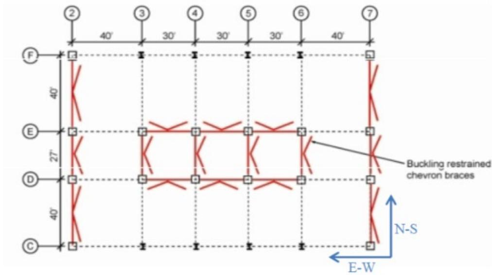
Figure 5 - Floor Plan for 20th, 30th, and 40th Floors
