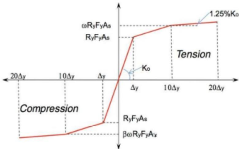
**General backbone curve for the nonlinear BRB element. The vertical axis represents force and the horizontal axis represents deformation.  $A_s$  = area of yielding steel core,  $K_o = A_s E / L$ ,  $E = 29,000 \text{ksi}$ ,  $F_y = 38 \text{ksi}$ ,  $R_y = 1.1$ ,  $\omega = 1.25$ ,  $\beta = 1.1$ , and  $L = 70\%$  of the brace length (using center-line to center-line geometry). Image courtesy of Dutta and Hamburger [2010].**
