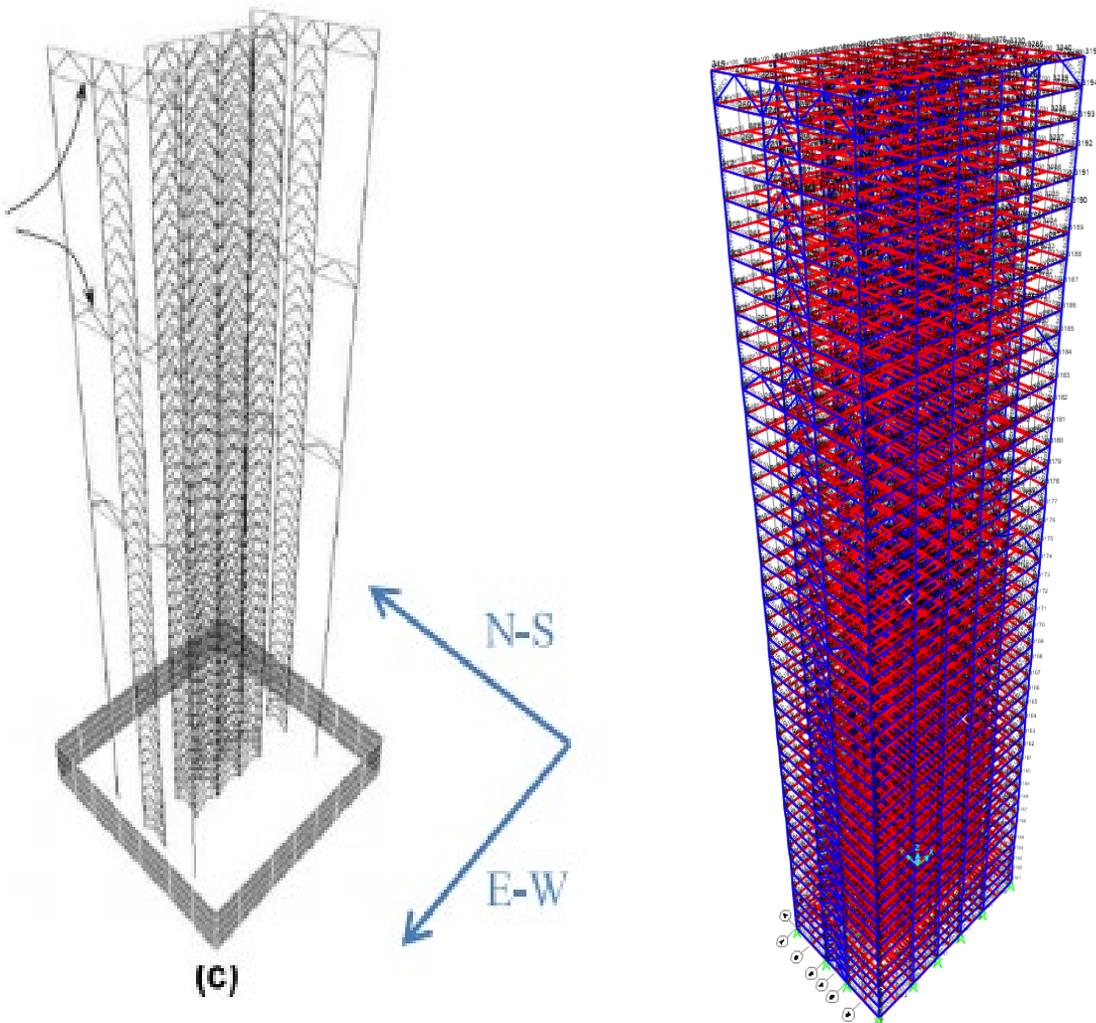
Figure 1 - Comparison of Skeleton Prototype Frame to SAP2000 Structure
