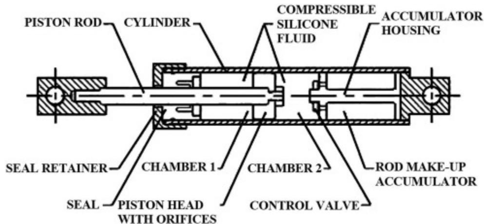
*Figure 4 - Model of a Viscous Damper*
